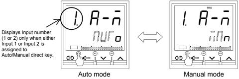
(The above figure is an image of Auto/Manual transfer of Input 1.)
