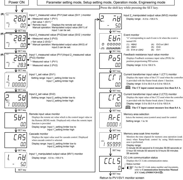
\* With the Setting change rate limiter when the set value is changed, the displayed set value changes according to the ramp-up/down rate.
