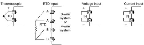
• For the 2-input controller, terminals 22 to 24 are allocated to Input 1, and terminals 19 to 21 are allocated to Input 2.
