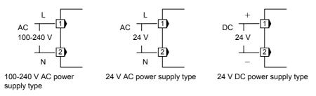
• The power supply types must be specified when ordering. Power supply voltage for the controller must be within the range shown below for the controller to satisfy the control accuracy in the specifications.
