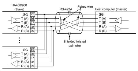
Maximum connections: 32 instruments maximum including a host computer
