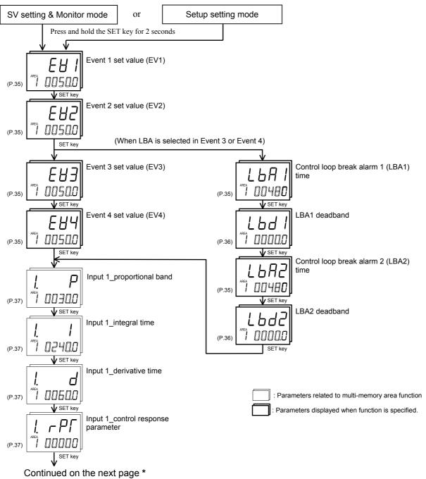
\*For 1-input controller: To Input 1\_setting change rate limiter (up) screen For 2-input controller: To Input 2\_proportional band screen
