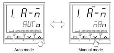
(The above figure is an image of Auto/Manual transfer of Input 1.)
