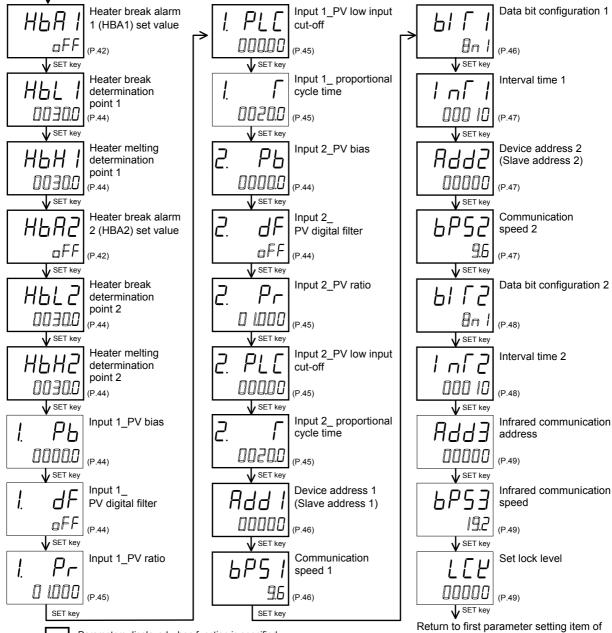
: Parameters displayed when function is specified.
