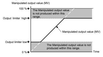
Output limiter is available for ON/OFF action.
