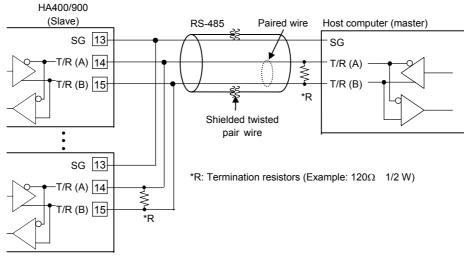
Maximum connections: 32 instruments maximum including a host computer
