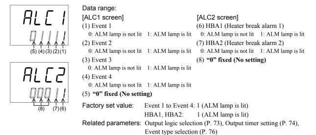
The alarm lamp is lit through the *OR* operation of Event 1 to Event 4, HBA1 and HBA2 each of which is set to "1: ALM lamp is lit."
