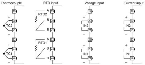
• The input types needs to be specified when ordering. The input types are as follows.
