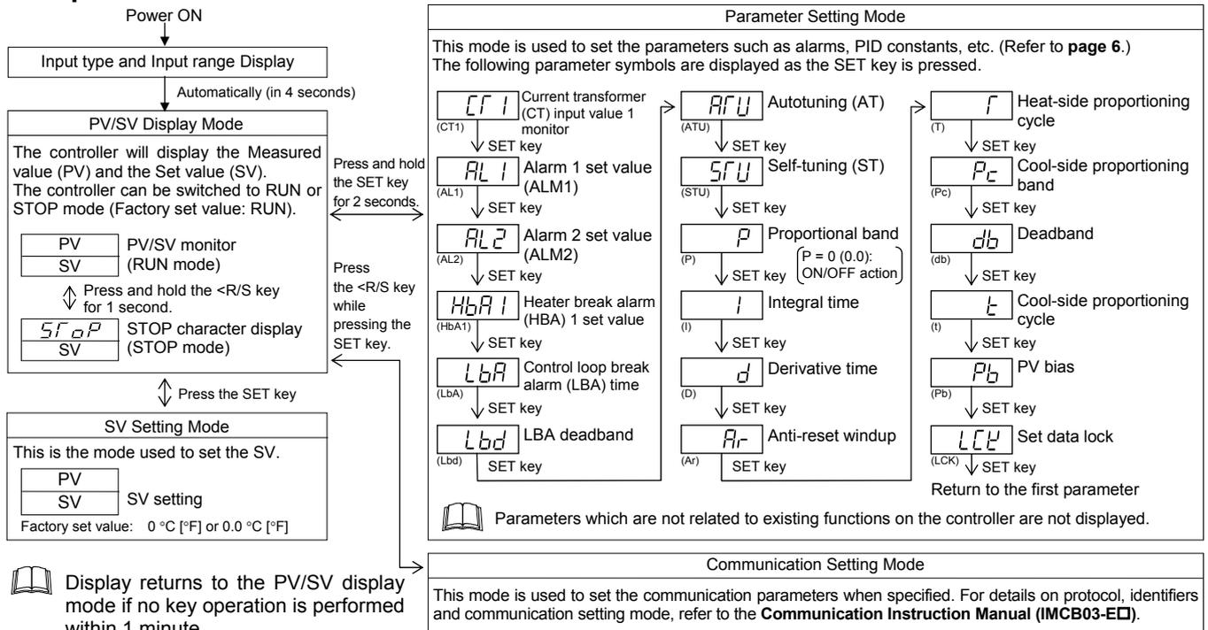
Display returns to the PV/SV display mode if no key operation is performed within 1 minute.
