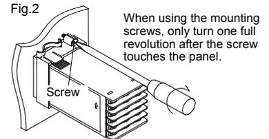
When using the mounting screws, only turn one full revolution after the screw touches the panel.
