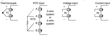
• For the 2-input controller, terminals 22 to 24 are allocated to Input 1, and terminals 19 to 21 are allocated to Input 2.
