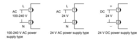
• The power supply types must be specified when ordering. Power supply voltage for the controller must be within the range shown below for the controller to satisfy the control accuracy in the specifications.
