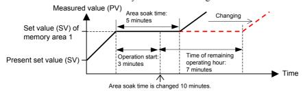
For the instrument with the 2-input specification, its area soaking starts based on the arrival at the memory area set value of Input 1 or that of Input 2, whichever later.
