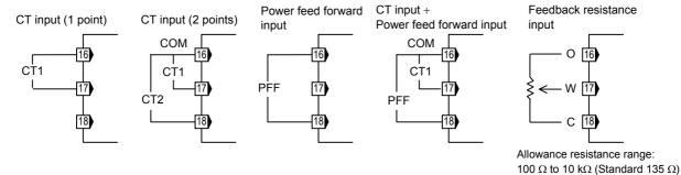
• CT input and Feedback resistance input are not isolated between measured input.
