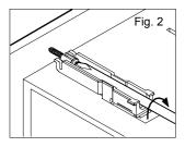
When the instrument is mounted, always secure with two mounting brackets so that upper and lower mounting brackets are positioned diagonally. (HA900/901 type)
