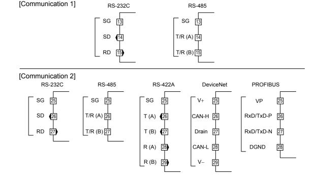
Example 1: Connection to the RS-232C port of the host computer (master)
