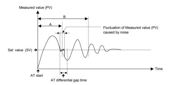
The factory set value of the AT cycle is 2 cycles.
