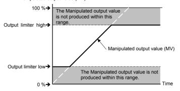
Output limiter is available for ON/OFF action.
